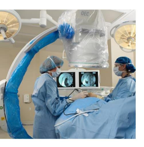
Mobile Fluoroscopic Imaging Systems to help guide minimally invasive surgical procedures
