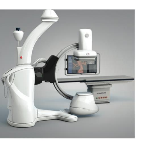
The Discovery IGS 730 angiography system brings both high-quality imaging and complete workspace freedom to the hybrid operating room to perform cardiac angulations without compromising detector coverage for endovascular procedures.
